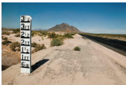
This gauge's vertical scale measures the depth of snow when it falls. It has a natural origin at the level of the road.
